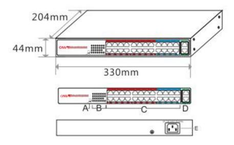
A.Multi-functional Switch B.Working LED Indicator
